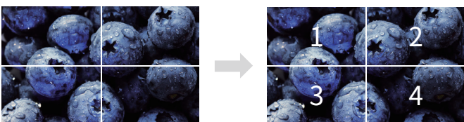
4K Square Division (SQD) : Quadrant based segmentation
