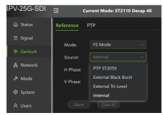
IP25G series monitor as a receiving and decoding device for remote data transmission, it is better to provide PTP network accurate master clock, so that the sending and receiving devices are uniformly locked in the PTP network accurate master clock, in order to achieve ultra-low delay data receiving and decoding output.
