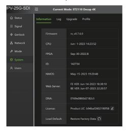
12) Select the Upgrade of the System option and upload a file to upgrade the firmware. System->Upgrade.
