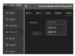
The IP25G series monitor supports the Network Group Management protocol of the IGMP V2/V3 version.
