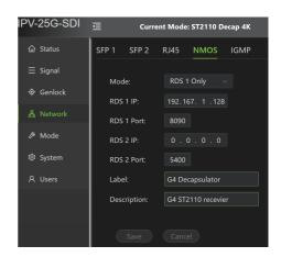
9) Select the IGMP of the Network option and adjust the parameters of each item. Network->IGMP.
